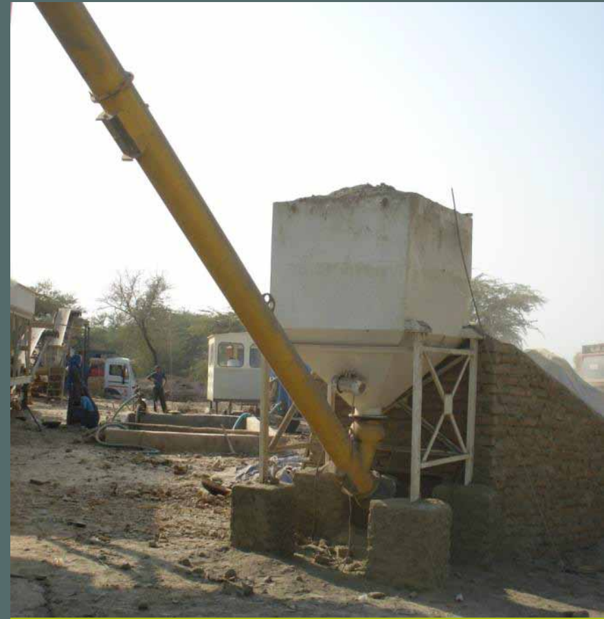
30 BAG CAPACITY CEMENT HOPPER WITH WAM (ITALY) MAKE SCREW CONVEYOR
