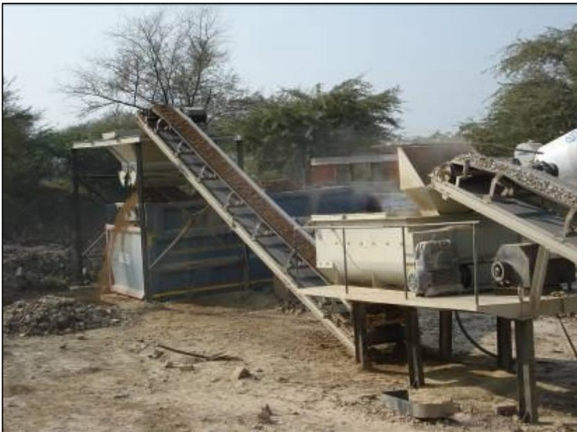
Truck loading will be by an inclined load out conveyor with belting equipped with a silo hopper with hydraulically operated cam shell gate to provide surge capacity when changing trucks & controls segregation in the mix.
