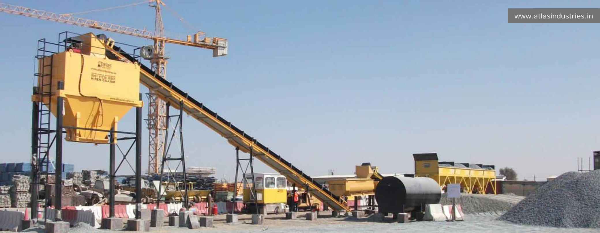
WET MIX PLANT WITH 25 T CAPACITY MIX MATERIAL STORAGE SILO
