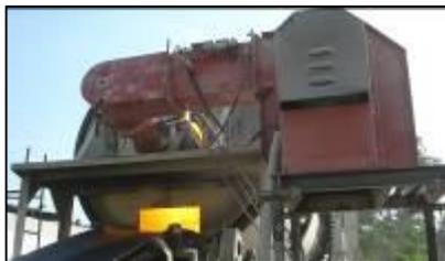
The burner of the dryer unit is capable of heating the aggregate to required temperature without any un burnt fuel or carbon residue on the aggregate and to reduce the moisture content of the aggregate to the specified minimum. The plant will be fitted with suitable type of thermometric instrument at appropriate places so as to indicate the temperature of exhaust gases, bitumen and mix.
