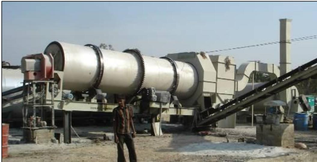
mounted exhaust fan and drive with a 20 HP (in DM 45), 25 HP (in DM 50), and 40 HP (in DM 60) electric motor. A frame mounted chamber at discharge end of drum has a special configuration to remove dust particles from the exhaust gas. A dust transfer screw at
