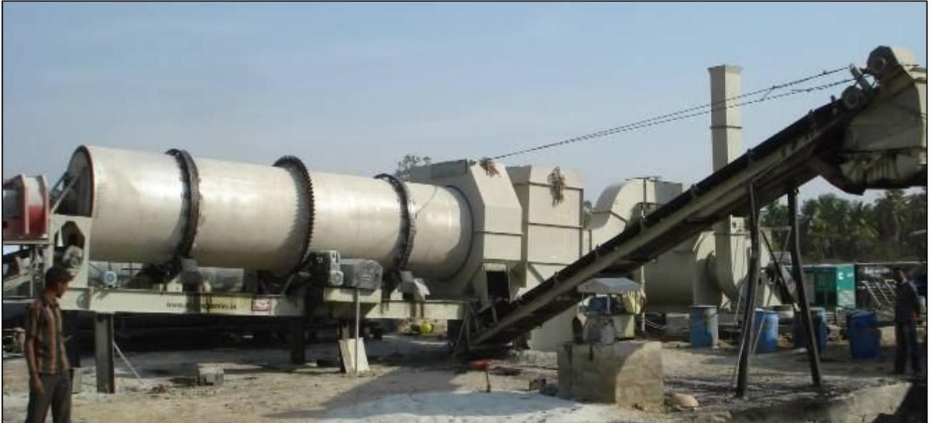
Loading of the trucks is done by an inclined load out conveyor which is provided with a heat resistant belt. Load out conveyor is equipped with a GOB hopper which is with a hydraulically operated cam shell gate in order to provide surge capacity when changing trucks and it also controls segregation in the mix.
