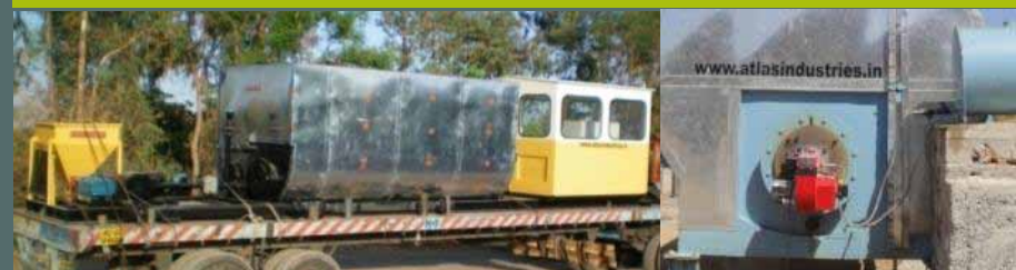
BITUMEN TANK WITH LIME FILLER AND CABIN
