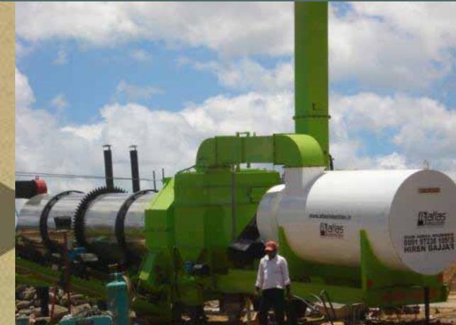
DRYER WITH WET DUST COLLECTOR
