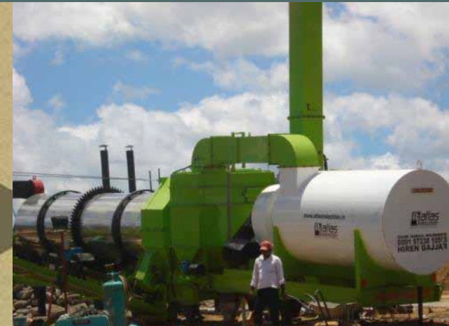
DRYER WITH WET DUST COLLECTOR
