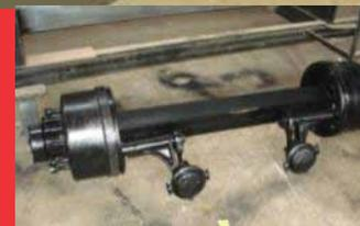
AXLE WITH PNEUMATIC BRAKING
