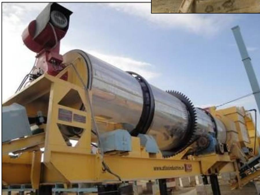
has a special configuration to remove dust particles from the exhaust gas. A dust transfer screw at the bottom of the chamber has a 2 HP electric drive to collect waste dust. The burner of the dryer unit is capable of heating the aggregate to required temperature without any un burnt fuel or carbon residue on the aggregate and to reduce the moisture content of the aggregate to the specified minimum. The plant will be fitted with suitable type of
