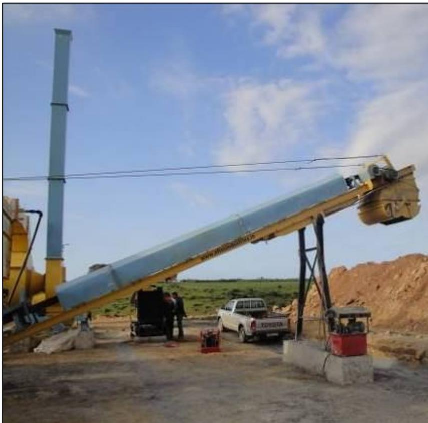
Loading of the trucks is done by an inclined load out conveyor which is provided with a heat resistant belt. Load out conveyor is equipped with a GOB hopper which is with a hydraulically operated cam shell gate in order to provide surge capacity when changing trucks and it also controls segregation in the mix.
